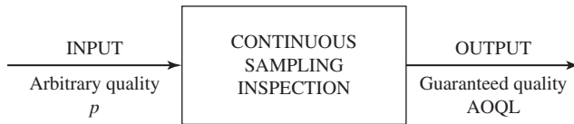
Figure 4.3 Black-box picture of a continuous inspection scheme as a method of guaranteeing outgoing quality.
